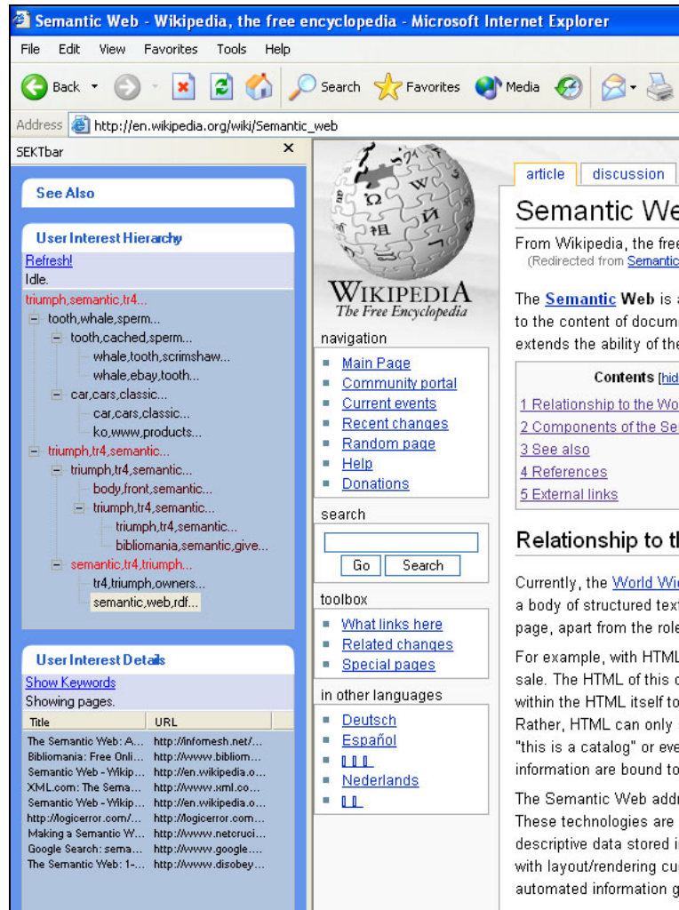
Figure 5. Screenshot of the system's GUI, captured after the user visited all the pages used for the demonstration in Section 4. Screenshot shows the topic ontology of the user's interests and the list of Web pages that corresponds to the semantic-web-rdf cluster. The user's most recent interest is highlighted with red color (the brighter the more relevant).
