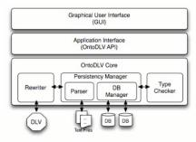
Fig. 1. The OntoDLV architecture
