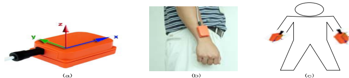
Fig. 3. (a) MTx accelerometer with 3-axis (b) MTx were attached (c) Accelerometers were mounted on wrist
