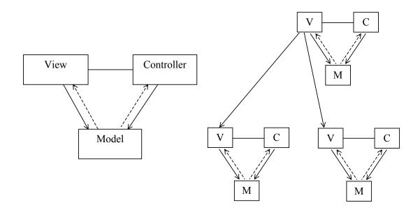
Figure 1. MVC and a hierarchy of MVC-triads
