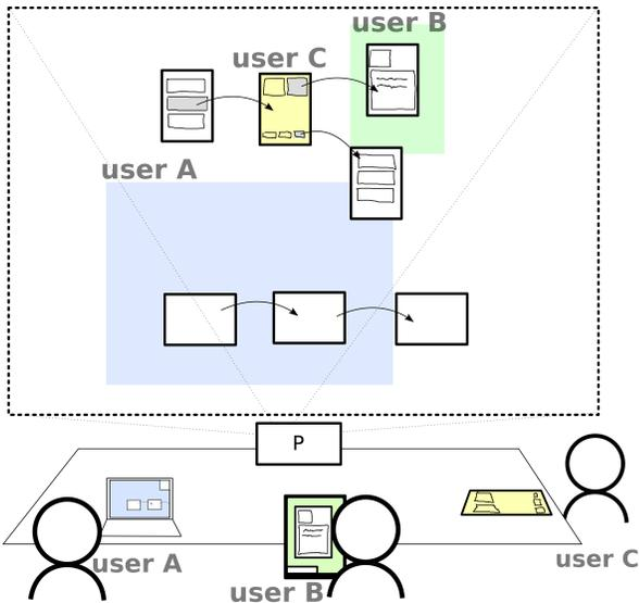
**Figure 1.** GAMBIT, a distributed sketching system. Left: users A, B and C collaborate in sketching activities, using respectively a laptop, a tablet and an interactive table. Right: 3 synchronized platforms in use for sketching.
