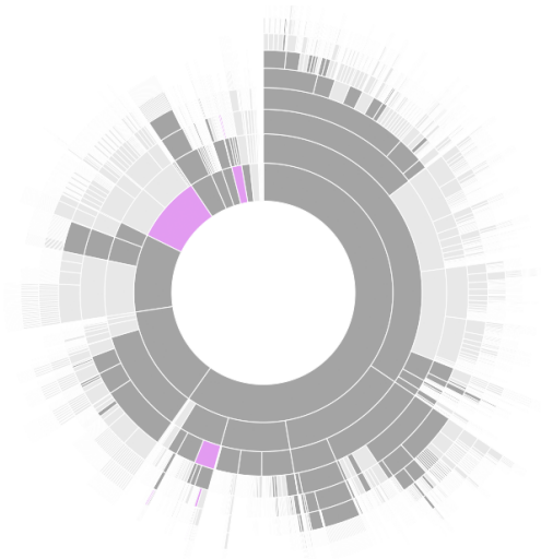
Fig. 3. A generic sunburst diagram: each block represents a node within a tree. The order and position of the blocks recreates the structure of the tree.
