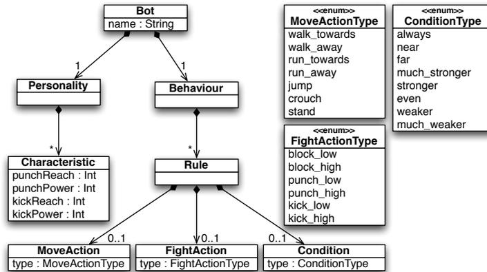
Fig. 2. Simplified metamodel for the FDL used to describe players in SAF.
