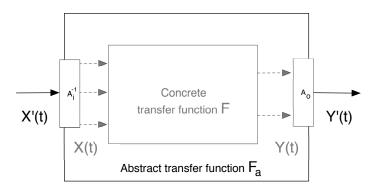
Fig. 5. Abstraction of a transfer function
