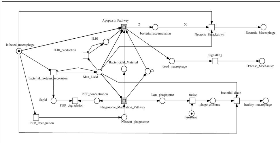
**Fig. 4: Petri Net of host-pathogen interaction at the top (root) level. The coarse transitions: *Phagosome\_Maturation\_Pathway* and the *Apoptosis\_Pathway* contain the second level of the model and are represented here by a double square.**
