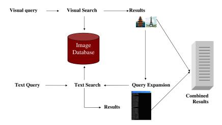
Figure 1: Architecture of the System
