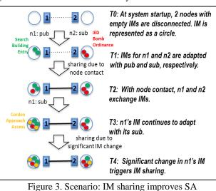
new data object encoded with IM elements to connected neighbors. Upon receiving neighbor's IM, the encoded information elements will be incorporated into the receiver's IM via the AIM adaptation algorithm.
