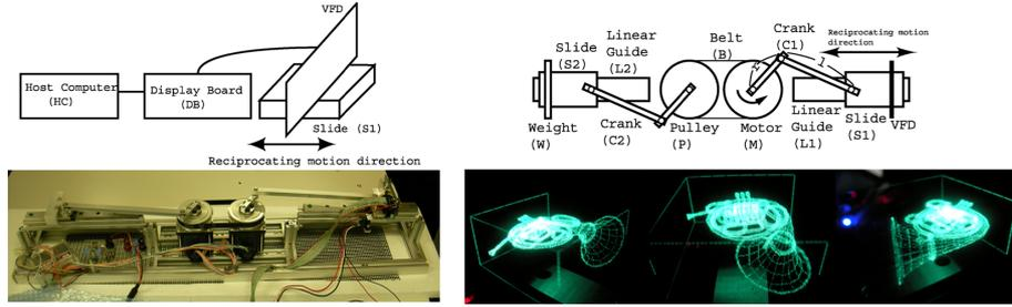
**Fig. 2.** (Above left) Schematic overview of our display, (Above right, below left) Schematic and photo of the reciprocating mechanism. (Below right) Sample 3D images on the display from three different viewpoints
