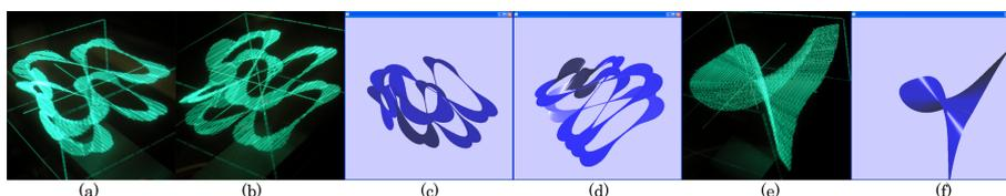
**Fig. 3.** (a) and (b) 3D images of tangent developable (TD1) on our display (from two different viewpoints). (c) and (d) 2D previews of TD1 on a PC screen. (e) 3D image of tangent developable TD2 on our display and (f) 2D preview of TD2 on a PC screen.
