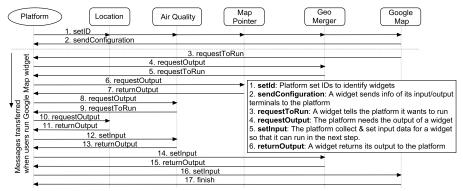
Fig. 5. An example of widget communication
