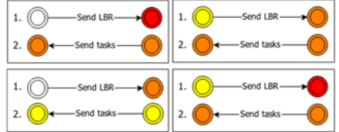
Figure 5: Possible states of host agents. Load balancing starts when the host agent is in Low or Low Average state. The numbers represent the stages of the Eager Worker algorithm
