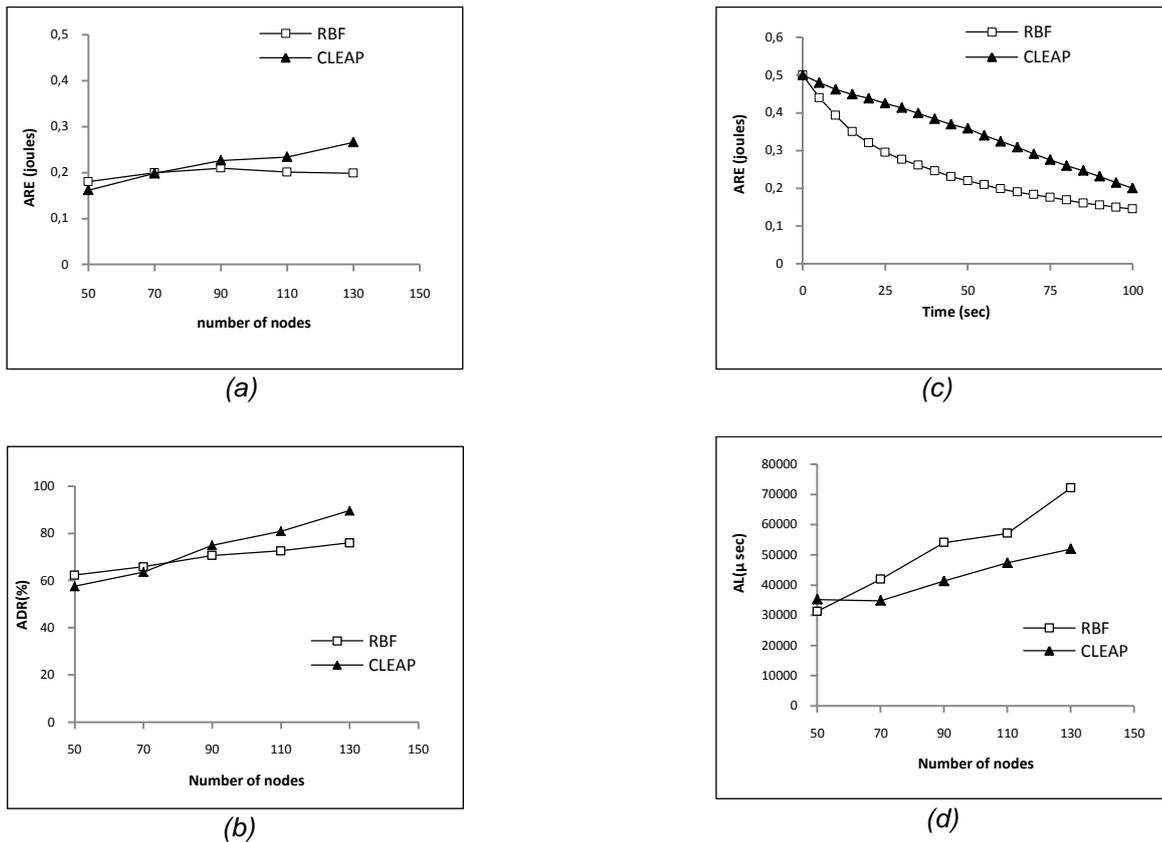
**Figure 2:** Simulation results. (a) Average residual energy vs. number of nodes; (b) average delivery rate vs. number of nodes; (c) average residual energy vs. time; (d) average latency vs. number of nodes
