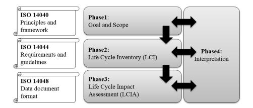
Fig. 3 ISO standards guideline of LCA
