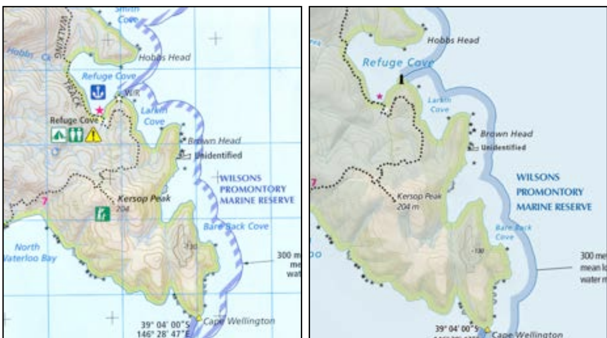
Figure 7: Left, portion of Wilsons Promontory print map (Spatial Vision, 2012). Right, portion of web map (Spatial Vision, 2012) using ‘design operators’ to calculate line weights, font sizes, symbols and colours. (Note that the print map is at 1:50,000 scale, whilst the web map is displayed at zoom level 14, approximately 1:36,000)
