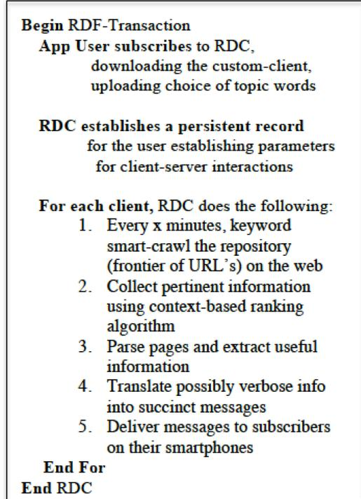
Figure 2: Top-Level Algorithm of System RDC
