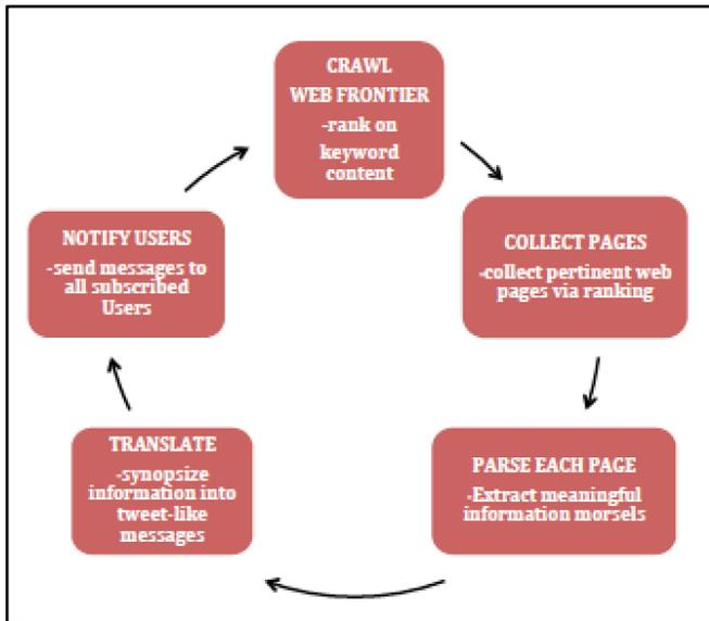
Figure 3: Software Components of RDC
