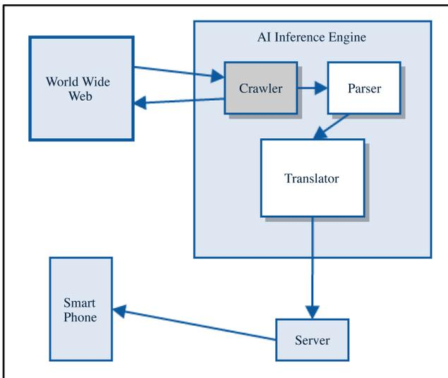
Figure 1: System Architecture of RDC
