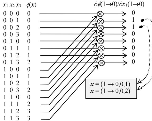
**Fig. 3.** Calculation of the Direct Partial Logic Derivative  $\partial\phi(1 \rightarrow 0)/\partial x_1(1 \rightarrow 0)$ .
