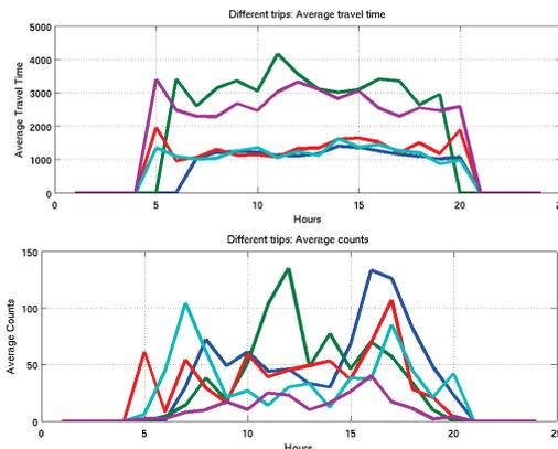
Figure 3. a) 5-top trips for one (origin, destination) pair in Nancy. b) The travel time and trip count distributions for top 5 trips.
