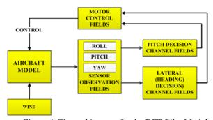
Figure 4. The architecture for the DFT Pilot Model.
