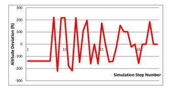
Figure 7.Pitch hold performance of the DFT pilot.
