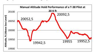
Figure 6. Manual altitude hold performance example from flight tests
