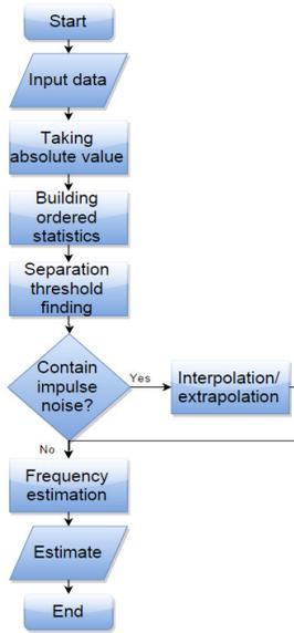
Figure 1: Flowchart of the frequency estimation process
