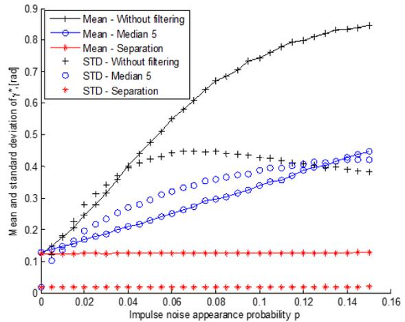
Figure 3: Comparison of precision indicators of frequency estimations for different filtration methods
