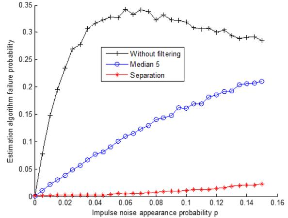
Figure 2: Comparison of algorithm failure probabilities for different filtration methods
