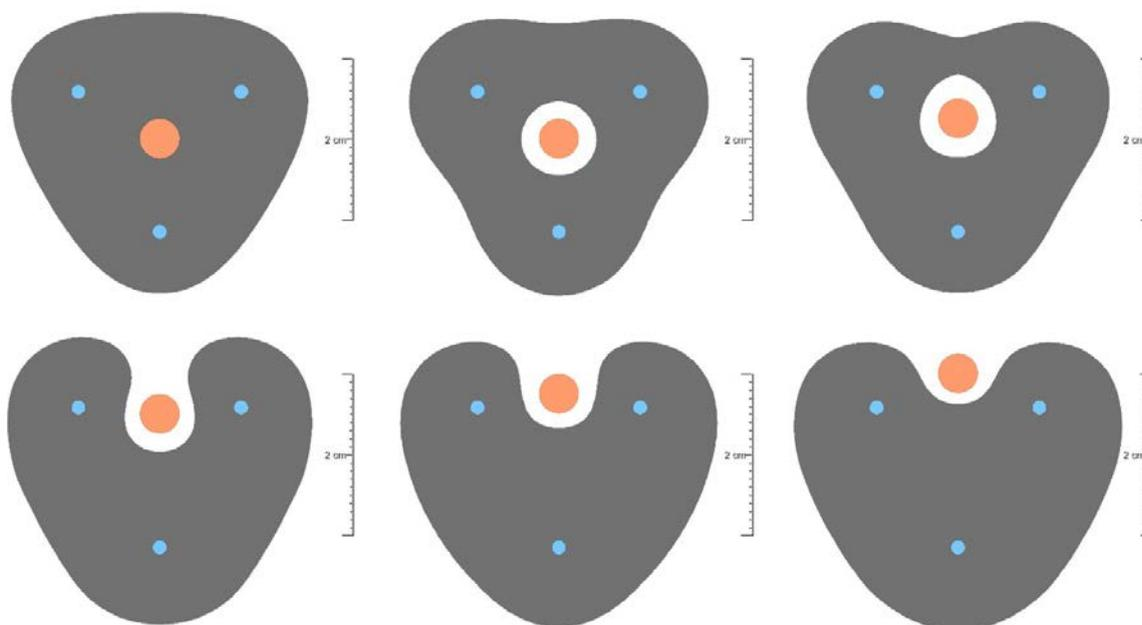
**Fig. 3:** Averaged ablation zone masks from ex-vivo experiments with three RF applicators and glass tube. From left to right upper row: ground truth, 0, and 2.5 mm distance of the glass tube to center of probes. From left to right lower row: 5, 7.5, and 10 mm distance.
