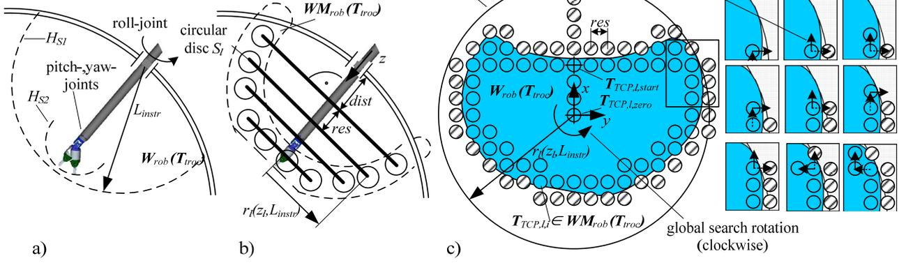
**Figure 3:** a), b) Geometric definition of the reduced MIRS-specific  $WM_{rob}(T_{troc})$ . c) Algorithmic calculation of the reduced MIRS-specific  $WM_{rob}(T_{troc})$ : All TCP poses  $\sum T_{TCP,i}$  which lie on the border of  $W_{rob}(T_{troc})$  within  $S_i$  are stored in  $WM_{rob}(T_{troc})$ . To identify the border, the search direction always rotates  $90^\circ$  clockwise if  $T_{TCP,i}$  is reachable and anticlockwise otherwise.
