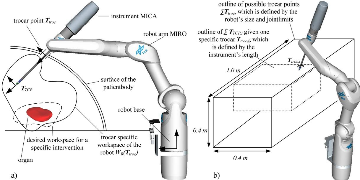
**Figure 1: a) The robot arm with the minimally invasive instrument MICA [4] inserted into the patient's body through a trocar. b) The outline of a specific  $WM_{rob,i}(T_{troc,i})$  compared to the outline of  $\Sigma T_{troc,i}$**
