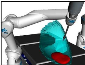
**Figure 4: Installation of one possible scenario: The surgeon checks on a screen if the desired trocar is suitable to reach e.g. a registered organ. To measure position of the trocar he uses the robot in the hands-on-mode.**
