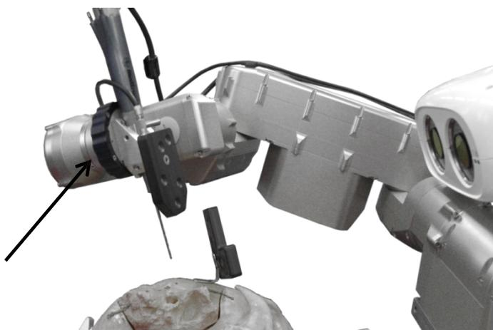
**Control:** As a final safety measure, the surgeon remains in control of the robotic system at all times. A 3-state dead man switch, consisting of wait, proceed and emergency halt conditions, ensure that the robot will not carry out the planned trajectory unless the surgeon is completely satisfied with the state of the procedure and allows the reversion to a standard mastoidectomy at any time.
