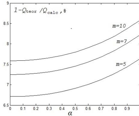
**Fig. 5.** Relation of error depending on asymmetry coefficient with  $m = 5, 7, 10$  and  $v_0 = 1$
