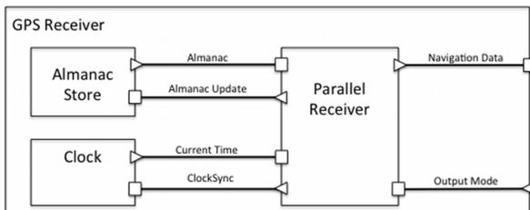
Fig. 2. A simple GPS receiver component.
