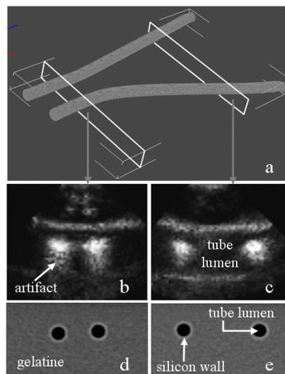
Figure 1: The physical vascular phantom includes two silicon tubes mimicking the blood vessels (a). (b) and (c) are two slices of the 3D USA data acquired with an US contrast agent. (d) and (e) are two slices of the CT volume.
