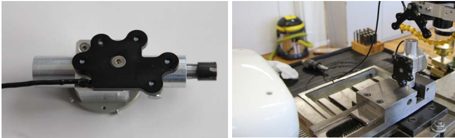
Figure 1: Developed sterilizable rigid body shield and robot tool (left). Set up for static positioning tests (right).
