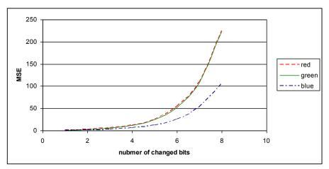
Fig. 8. – Dependency graphs of MSE distortion and the quantity of changed bits for the light container
