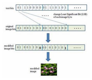
Fig. 1. – The scheme of LSB method
