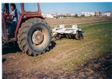
Fig. 1. Electrical resistivity instrument (VERIS)
