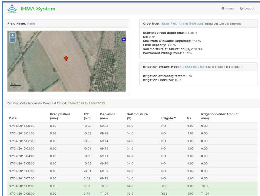
Fig. 10. Detailed irrigation report module of the IRMA\_SYSTEM.
