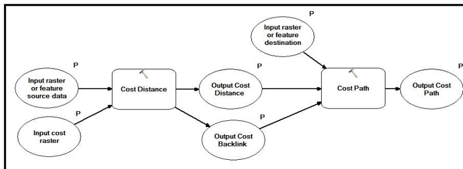
Fig. 6. Model for determining optimal path (cost path)
