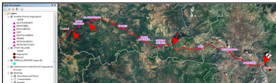
**Fig. 5.** Marked points with steep slope (> 60%) over the entire length of the route Orchard – Argyropouli
