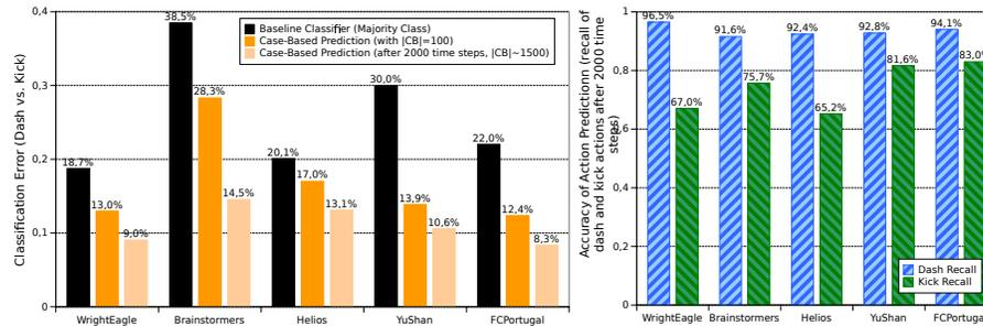
**Fig. 3.** Left: Case-based prediction of the type (dash or kick) of the next low-level action for opponents from different teams. Right: Recall, i.e. share of dashes that were correctly predicted as dashes and kicks that were correctly predicted as kicks.
