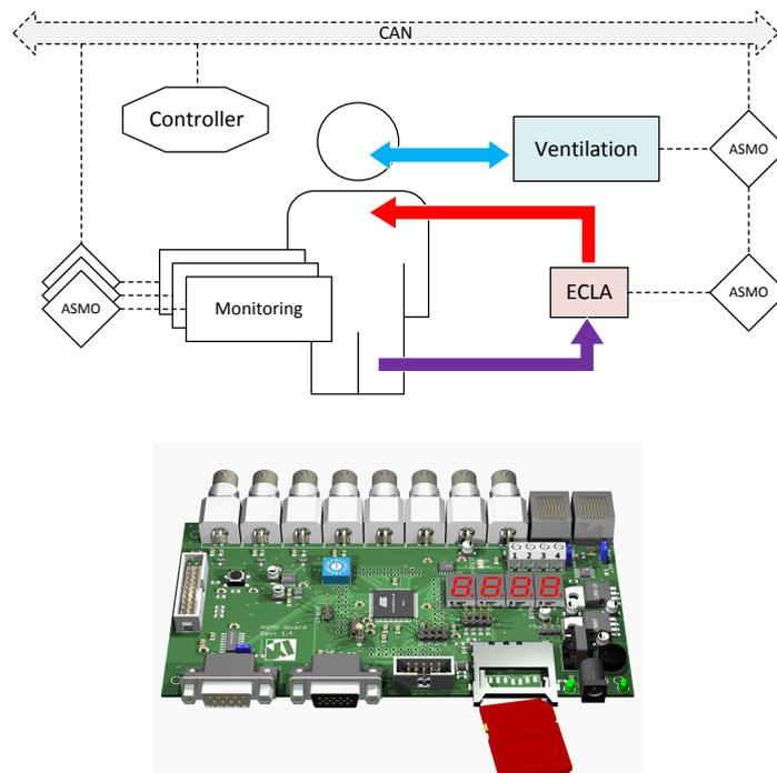
Fig. 1: Automated ARDS therapy setup and ASMO node hardware design [St13]
