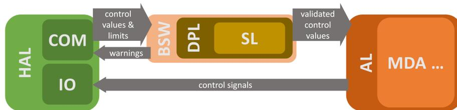
Fig. 3: Safety layer in ECLA-VENT
