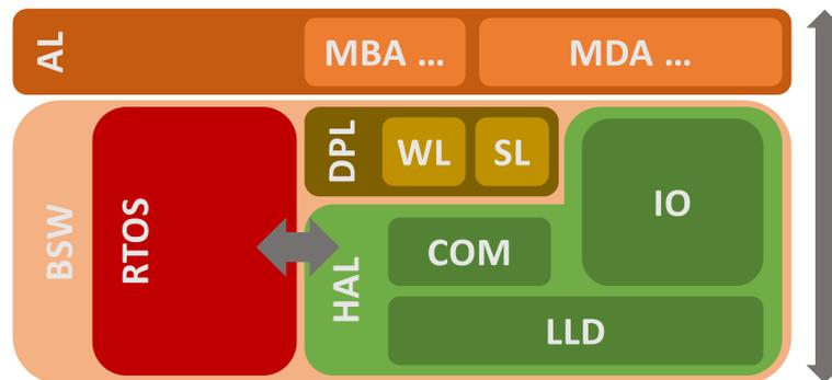
Fig. 2: Software architecture in ECLA-VENT
