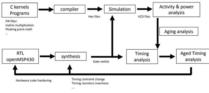
Fig. 2. Workload dependent Aging analysis Flow
