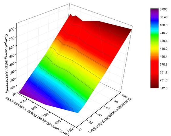
Fig. 4. Output Rising Delays when SP(0)=0.9.
