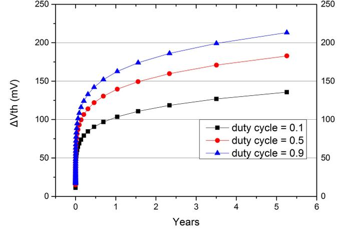
Fig. 1.  $V_{th}$  degradation for different duty cycles.
