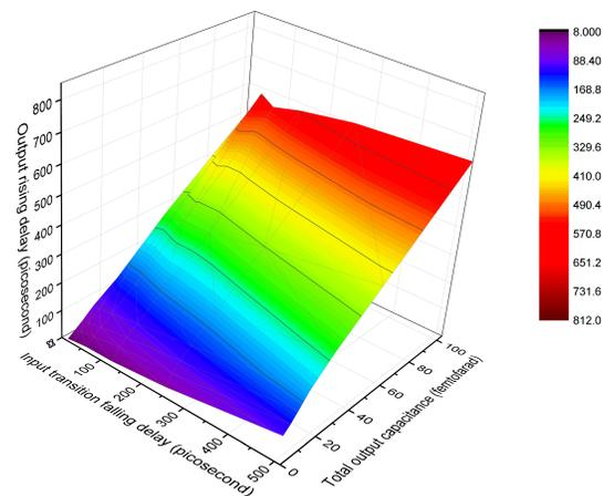
Fig. 3. Output Rising Delays when SP(0)=0.1.
