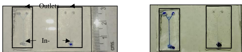
Fig. 6. (a) Fabricated coated and non-coated microchannels before sample introduction, (b) coated and non-coated channels after blue colour solution sample introduction. As a result of gel coating the sample flowed through the coated channel without any external field applied
