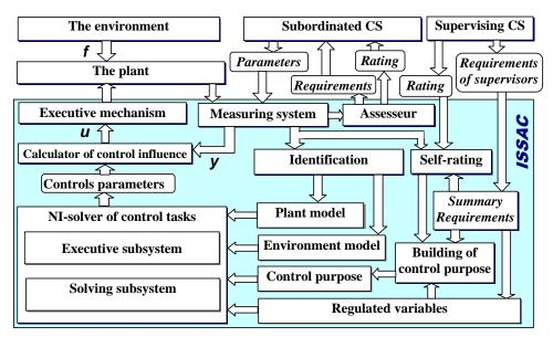
Fig.2. The diagram of the intellectual self-organized system of automatic control
