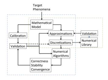
Fig. 2. Schematic of prototype development when the model needs more than one component. Here one component needs a new numerical algorithm, while the other component is using a library. Discretization is the same.
