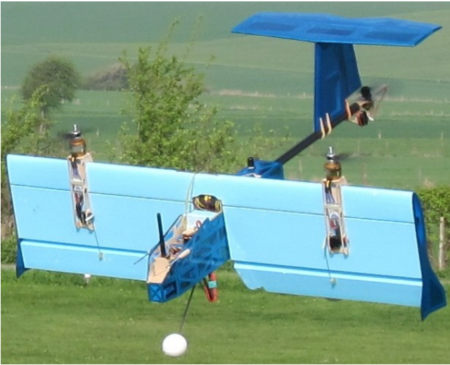
Fig. 2. Tilt-wing UAV after take-off in vertical flight. Two main engines at the wing yield thrust for take-off, while the tail rotor stabilizes pitch
