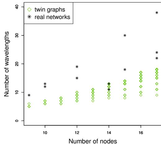
Figure 2: Number of wavelengths given the number of nodes for twin graphs and real-world networks.
