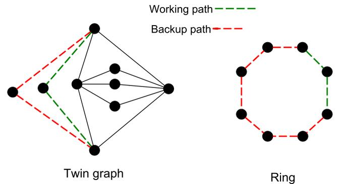
Figure 1: After any single node removal in a twin topology, there is always a backup path which has the same length of the working path. In a ring topology, the backup path can be much larger than the working path, since the length of both these paths have always to sum up the length of the ring.
