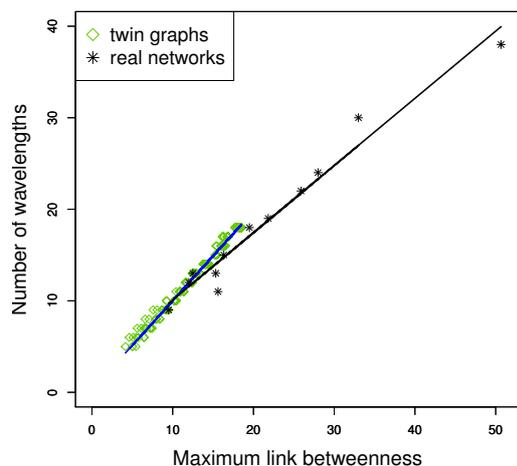
Figure 3: Number of wavelengths given the maximum link betweenness for twin graphs and real-world networks.
