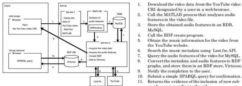
Fig. 2. Structure of the system
