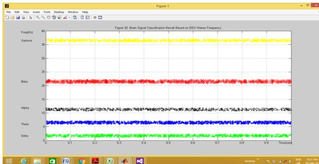
**Figure 4: Classification of EEG Signals into Five Distinct Frequency Waves**
