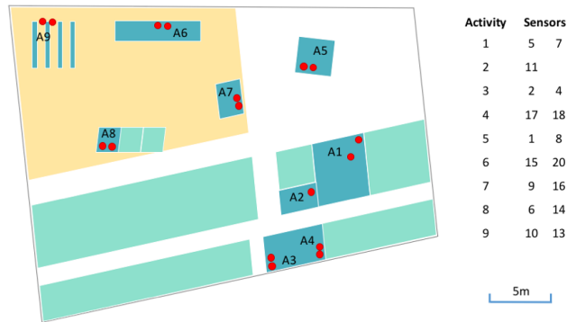
Fig. 4: Case study in Aalto University: sensors setting for process measurement
