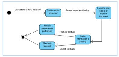
Figure 3. State machine diagram for the reactive version
