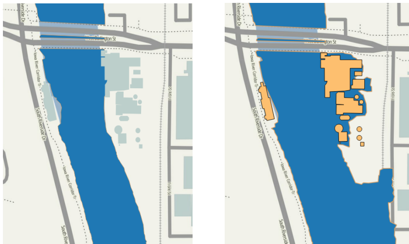
Fig. 2. Geo-visualization of space-time events. River flood stage increasing to 639.2ft (left blue) and again to 644.2ft (right blue). Hydrologic Lab and Power Plant flooded (right orange).
