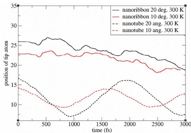
Fig. 4. Position of tip atom in the oscillation plane as a function of time for the first 3000 fs: nanoribbon vs. nanotube
