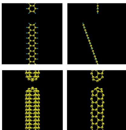
Fig. 1. Hydrogen passivated nanoribbon (top) and capped nanotube (bottom)
