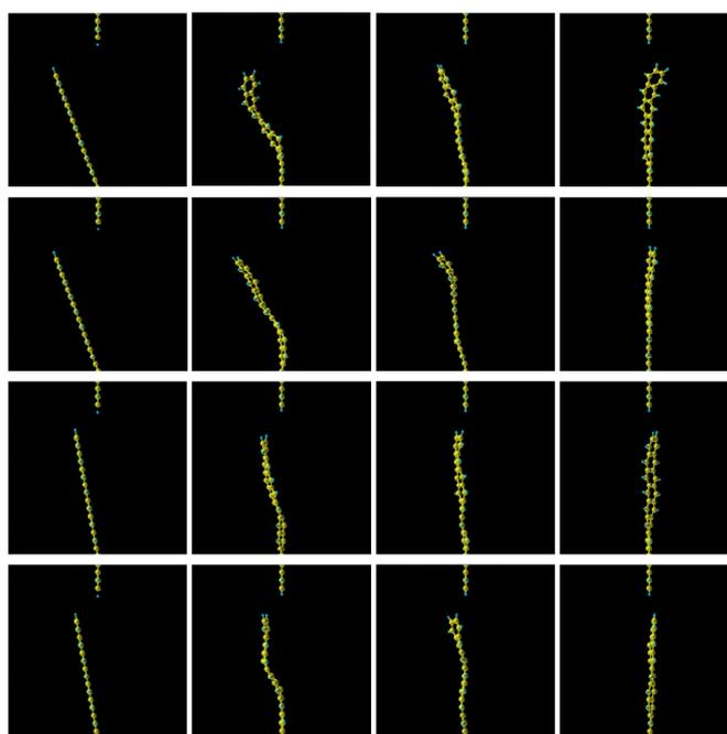
Fig. 2. Snapshots from the MD simulation of C nanoribbon taken at 0, 1000, 2000, 3000 fs - from left to right - at initial deflections of 20 degrees (for 300 and 150 K) - top two sets, and 10 degrees (for 300 and 150 K) - bottom sets
