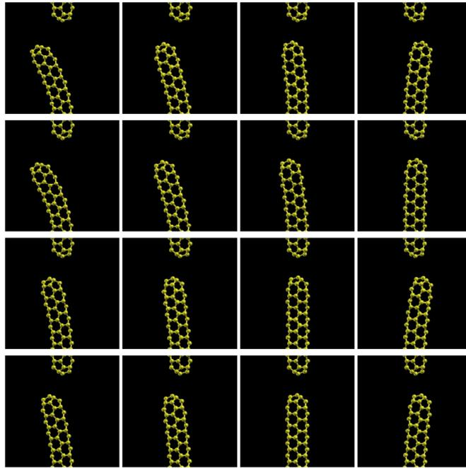
Fig. 3. Snapshots from the MD simulation of C nanotube taken at 0, 200, 400, 600 fs - from left to right - at initial deflections of 20 degrees (for 300 and 150 K) - top two sets, and 10 degrees (for 300 and 150 K) – bottom sets
