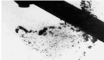
Fig. 2. X-ray pattern of steel screen penetration (thickness 6 mm) by a projectile of tungsten alloy 0.4 cm in diameter and elongation of 10 at an angle of 60 degrees at a speed of 2764 m/s.
