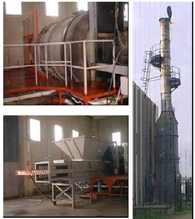
Fig. 2. Primary chamber, mechanical loader and reheat.
